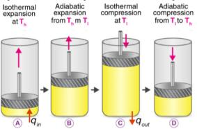
In (a), the process is reversible isothermal gas expansion. In this process, the amount of heat absorbed by the ideal gas is  $q_{in}$  from the heat source at a temperature of  $T_h$  The gas expands and does work on the surroundings.
